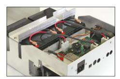
**6** Make sure the battery tray is seated on a flat and stable surface.
